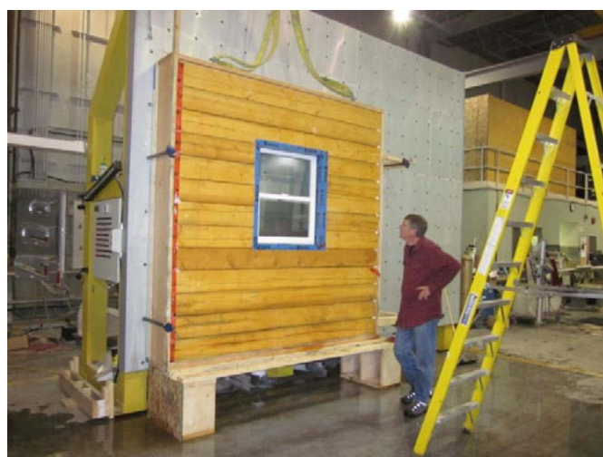
A log wall is being tested in a laboratory as part of a project to grow B.C.'s log home and timber frame industry.
