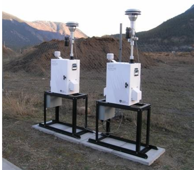
Airborne particulate monitoring instruments near the T'it'q'et First Nation in Lillooet (left) and the Mobile Air Monitoring Laboratory (right)
